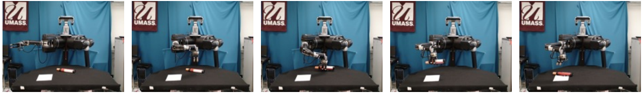
Fig. 4. The robot performing a top grasp on the object and placing it on the goal.
