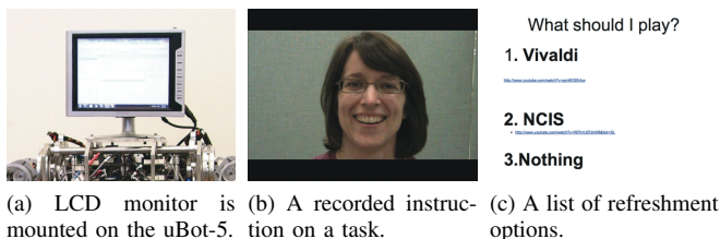
Fig. 4: Before each exercise task, the recorded instruction and demonstration are displayed on the LCD monitor which is mounted on the uBot-5. During the break between exercises, a short video clip is displayed based on the patient’s choice.
