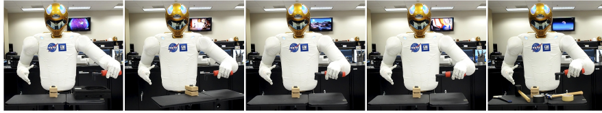
Fig. 6 Corner case initial settings for mating the socket with the bolt. Note that in the 3rd and 4th image the in-hand ratchet positions are different.
