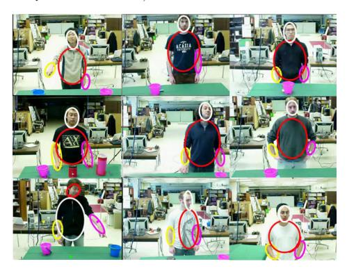
**Figure 4.14.** Examples of multi-body tracking of humans using the learned affordance human catalog model. Note that the probabilistic approach enables the algorithm to maintain a robust track of the human under partial occlusion or unstable feature conditions (as shown in the second picture in the top row).
