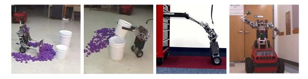
Figure 6.5. The uBot performing plowing, stacking, pushing, and throwing tasks.
