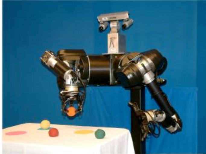
Figure 3.6. Dexter is a bimanual upper-body humanoid.
