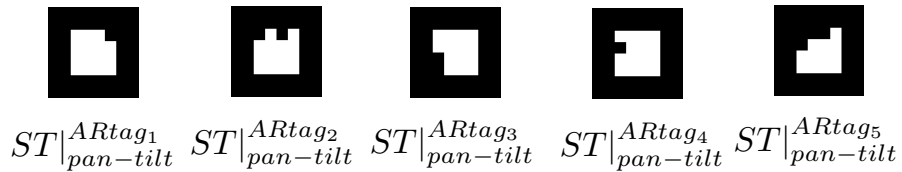
Figure 4.4. The set of visual actions being used to model the objects. The visual actions track a set of ARtag features.
