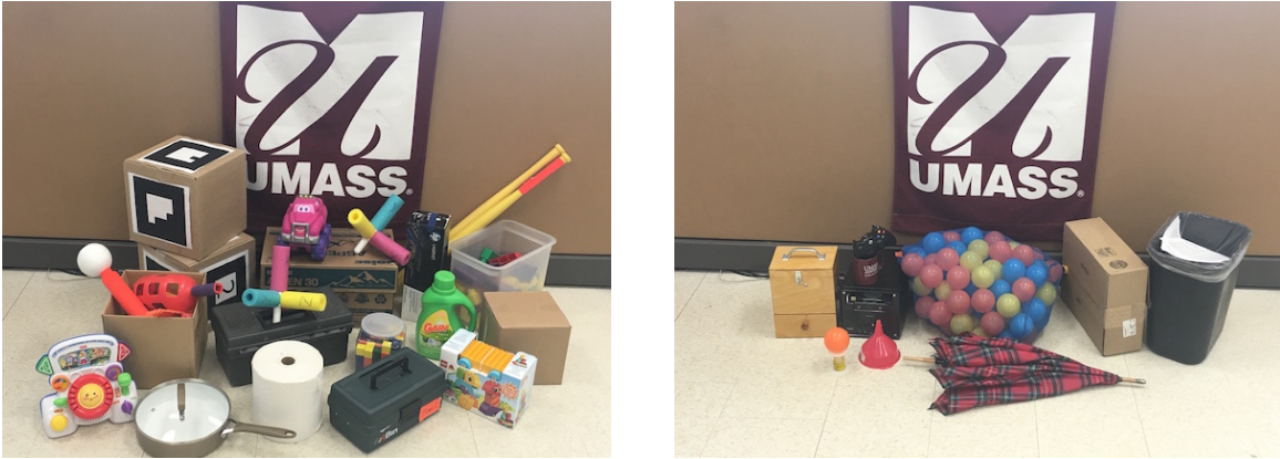
Fig. 6: Training set (left) and test set (right). Training set consists of twelve varying objects with a number of distractors such as blocks, bats, and toys. Two of the twelve objects were from the YCB grasping dataset. The test set consisted of ten novel objects with half being physically not graspable given the properties of the object and the robot.
