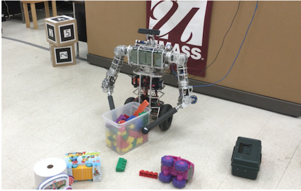
Fig. 1: Self-supervision: uBot-6 self-labels its own grasp experiences for training using closed-loop controller (motor unit) feedback.
