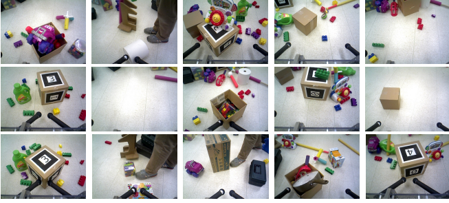
Fig. 4: Failed grasps: Selected grasp examples consisting of RGB (left) and depth (right) that resulted in grasp quiescence or failure.
