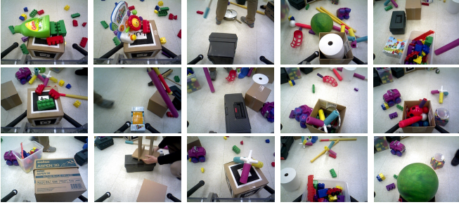
Fig. 3: Successful grasps: Selected grasp examples consisting of RGB (left) and depth (right) that resulted in grasp convergence.
