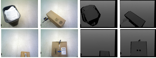
Fig. 8: Incorrect Prediction: Selected incorrect prediction examples consisting of RGB (left) and depth (right) that were taken before the grasp action started. The images in the first row depicts the case where the robot has predicted a convergent grasp, but in reality resulted in quiescence. The second row shows the case where the robot predicted a quiesced grasp outcome, but the grasp resulted in convergence. The bottom rightmost panel illustrates a cardboard box that is tilted with respect to the horizontal plane.
